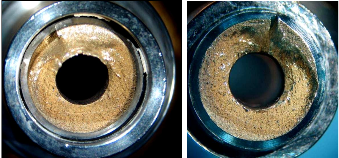
Figure 8- View of sample 1-2(Left) and sample 1-2-T(Right) fracture faces, consistent with brittle fracture over approximately 90% of the cross section followed by a shear lip
