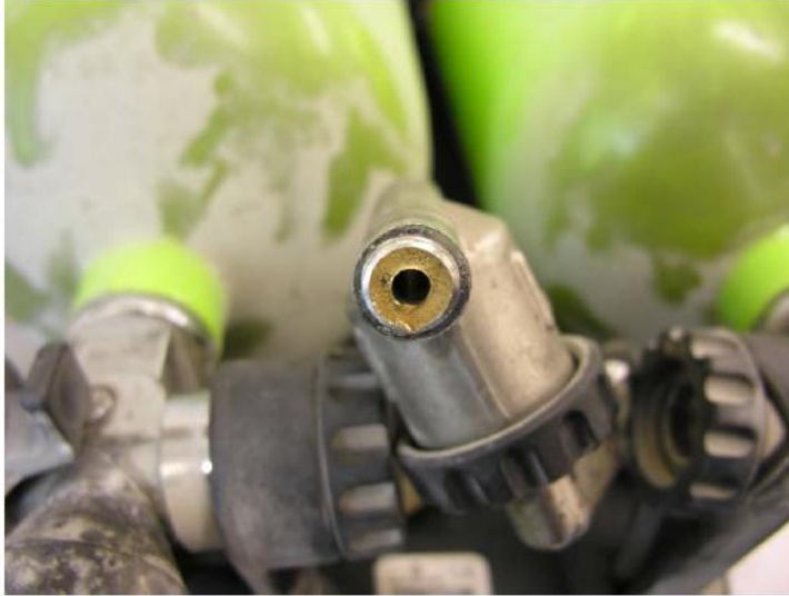
CABA unit showing broken connection
