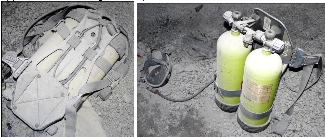
Figure 1- Showing a self-contained compressed air breathing apparatus combined of two air bottles, a T-piece which connects the bottles and a backpack.
