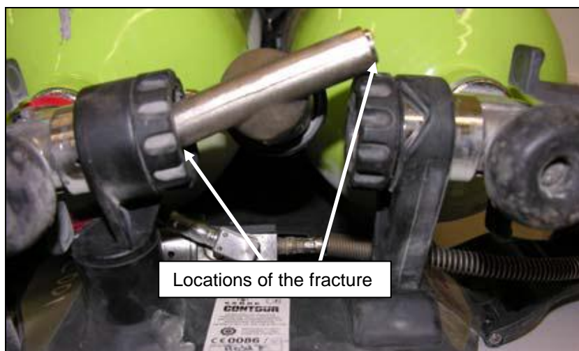
Figure 4- General photo of the failed CABA unit from 5/1/2011 showing the location of the fracture.
