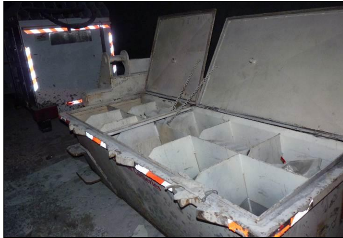
Figure 2- showing the container for SCABA units.
