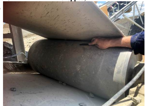
IMG_1321: RHS of CV2 Tail pulley looking towards Screen 1. Rocks on belt. Cuts in belt and indentation marks on tail pulley.
