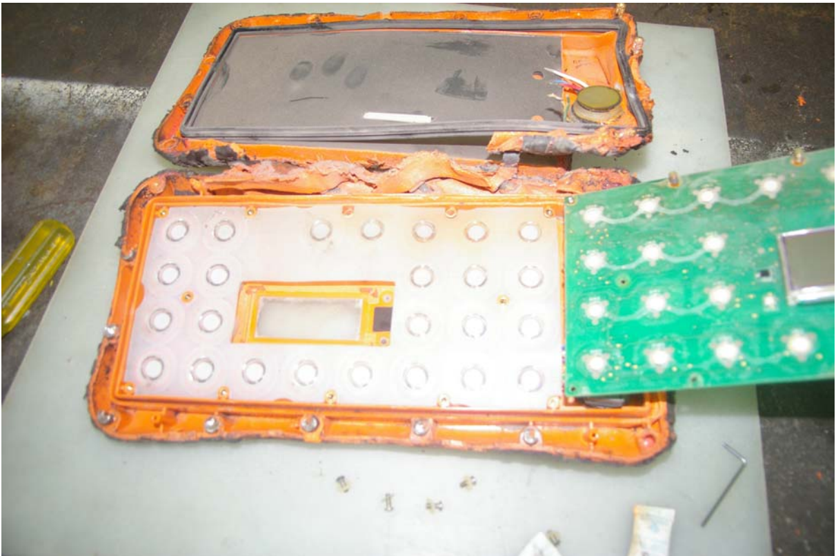
Photo 7 – keypad, membrane & circuit board separated
