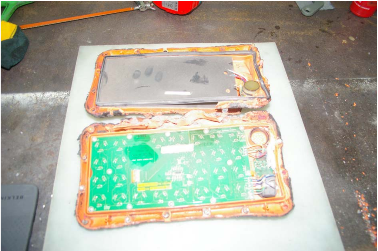
Photo 4 – control unit opened, showing circuit boards
