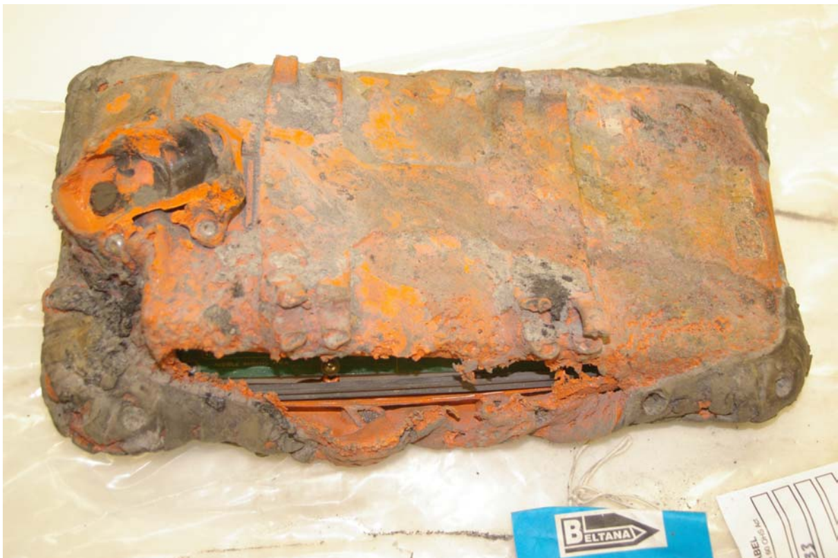
Photo 2 – reverse side of control unit, showing cable entry
