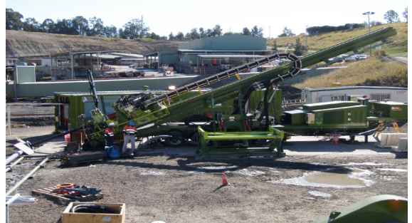
Drills +200m/day, capable of 300m/day, achieved 1300m/12hrs tripping
