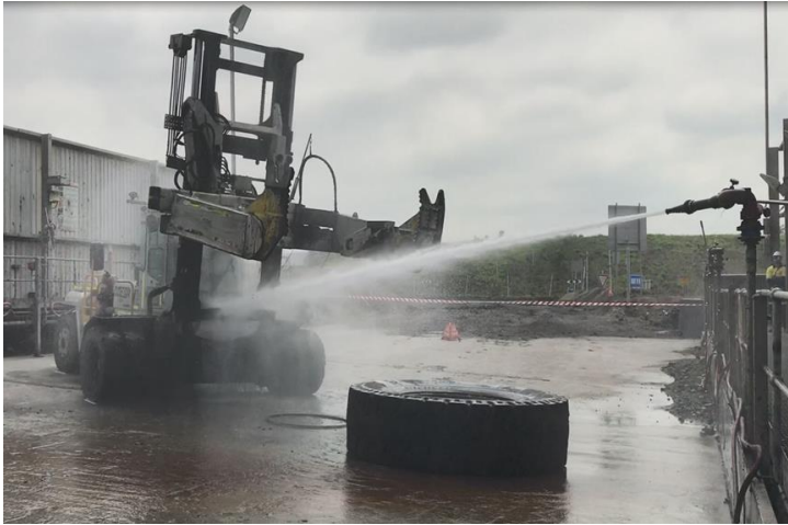
Figure 26 Photo of tyre location after falling from grabs during test 1
