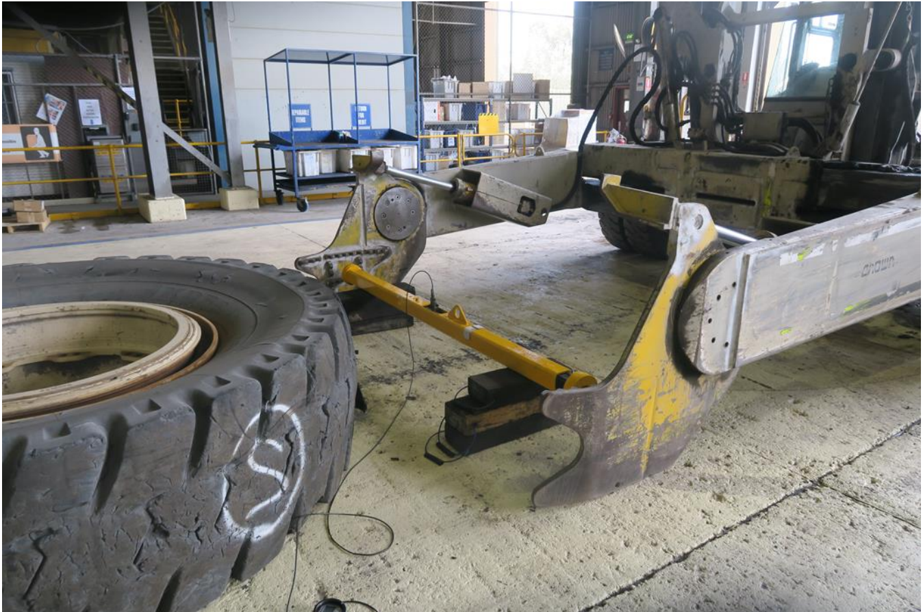
Figure 14 Clamp force pressure test on THL001 by Cascade
