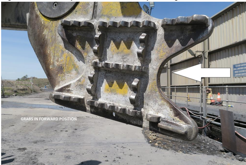
Figure 25 Grabs on tyre handler as found by investigators
