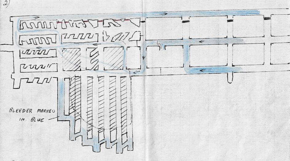
ON THE AFTER MOON OF JUNE 24TH MYSELF AND TWO MINERS ERRECTED BRATTICE (MARRED IN RED) ACCROSS THE HOLES WHICH HAD BEEN PUNCHED FILLAR. TO RETURN. THIS CLEARED THE CH4 FROM THIS AREA. THE DIRECTION OF THE. AIR. FLOW. MARKED IN BLUE, NO WENTLATION FLOWED THROUGH THE BLEEDER SYSTEM POWN THE BOTTOM. A ROAD WAS REGULAED TO BE DRIVEN DOWN AND A HOLE PUNCHED THROUGH TO THE BLEEDER TO LET IT SERVE ITS PURPOSE. IN. THE MEANTIME A FALL TOOK PLACE BETWEED THE BELT ROAD AND
