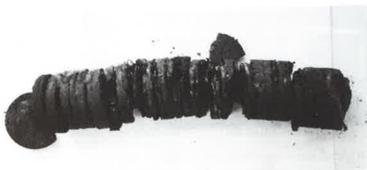
Fig. 4 Discing in coal core from the Bulli seam (465 m depth, 98% CO 2 , 18 m 3 /t)
