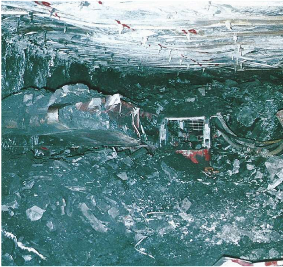
Mining machine almost buried with coal from a fatal outburst at Tahmoor Colliery
